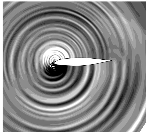
Fig. 18 The acoustic pressure field solved by the source-driven APE with a hard wall condition.
